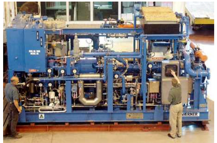
Fig. 6-Photograph off 24 RST skid package for offshore evaluation program.
