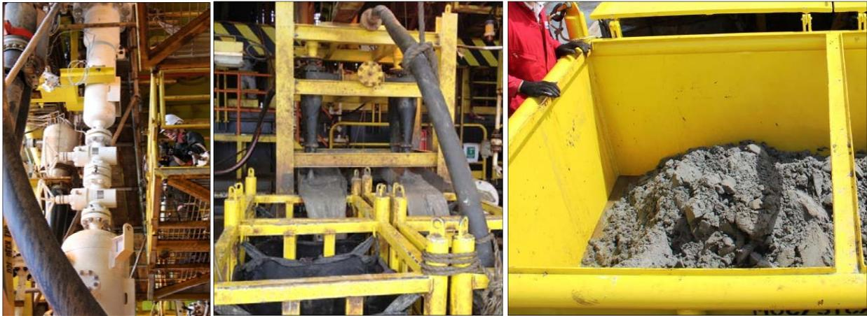
Figure 6 – (left) 1500# wellhead desander integrated into the deepwater spar well bay, (middle) solids collection and dewatering station, and (right) collected solids transported by skip to landfill disposal.
