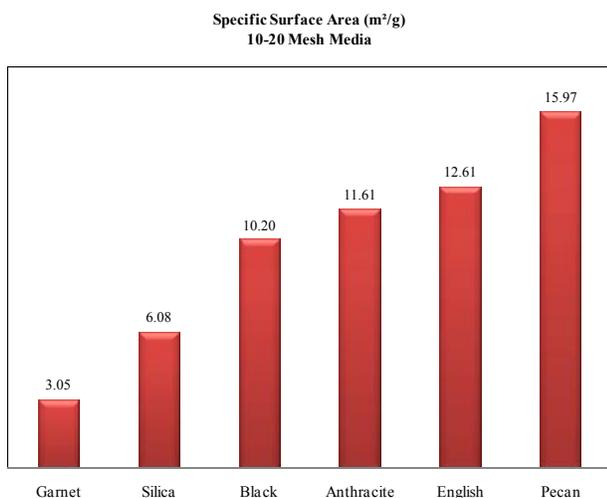
**Figure 3.** Specific surface area (m<sup>2</sup>/g) of six filter media with 10-20 mesh size.
