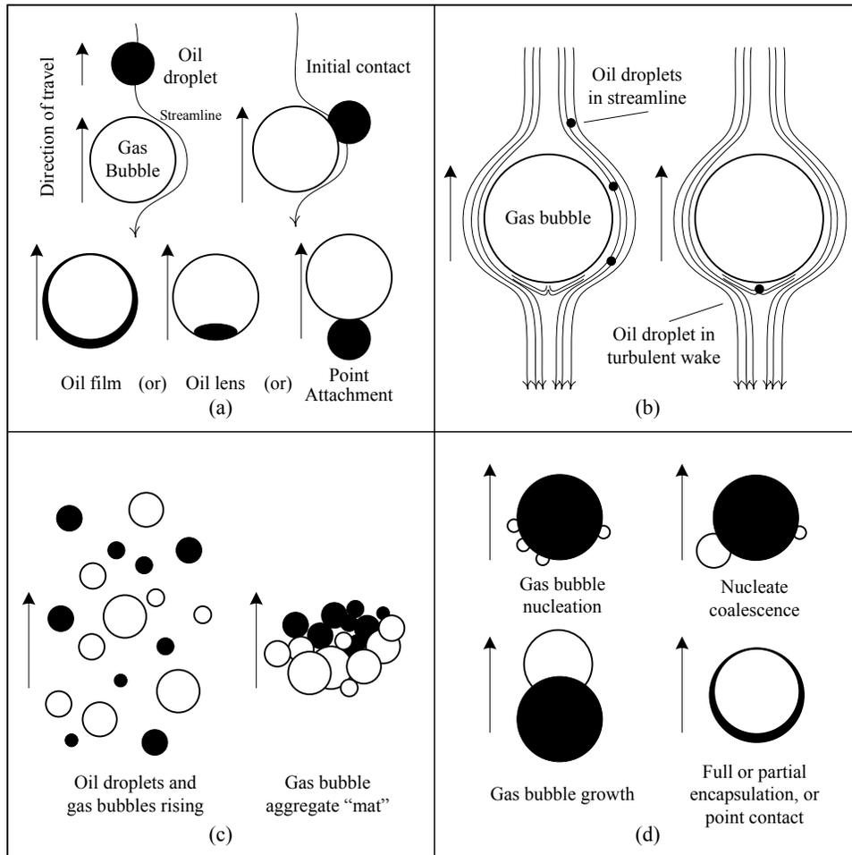
**Figure 6. Mechanisms for gas bubble capture of oil droplets suspended in water: (a) direct impingement with full or partial encapsulation by chemical adhesion, (b) hydrodynamic capture of oil droplets in the wake of a rising gas bubble, (c) clustering of gas bubbles to form a buoyant mat, and (d) gas bubble nucleation, coalescence, and growth on the surface of an oil droplet to result in full or partial encapsulation**
