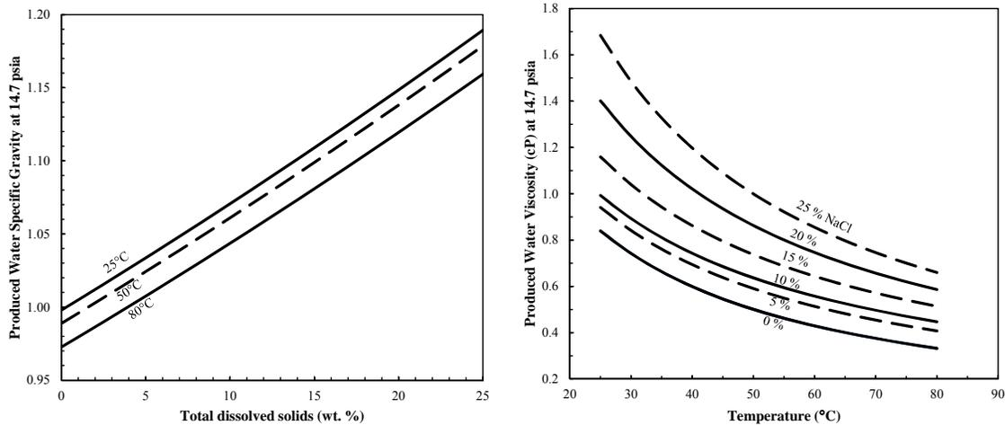
**Figure 2. (left) The effect of dissolved solids (as salinity) and temperature on the specific gravity of produced water (data from McCain 1990 and Street et al. 1996) and (right) the effect of salinity and temperature on the viscosity of produced water (data from McCain 1990).**
