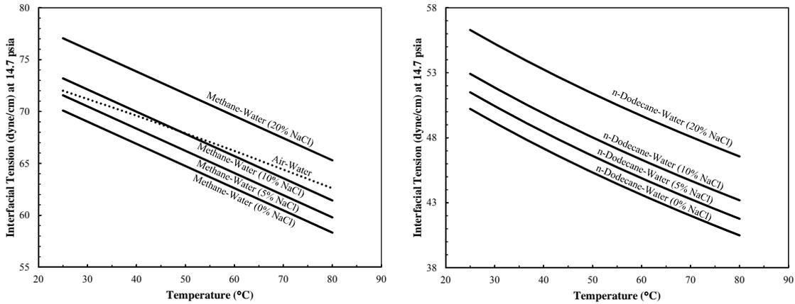
**Figure 3. (left) The effect of dissolved solids (as salinity) and temperature on the interfacial tension between methane and water at ambient pressure (data from Jennings and Newman 1971; Street et al. 1996; Argaud 1992) and (right) the effect of salinity and temperature on the interfacial tension between n-dodecane and water at ambient pressure (data from Street et al. 1996; Argaud 1992).**
