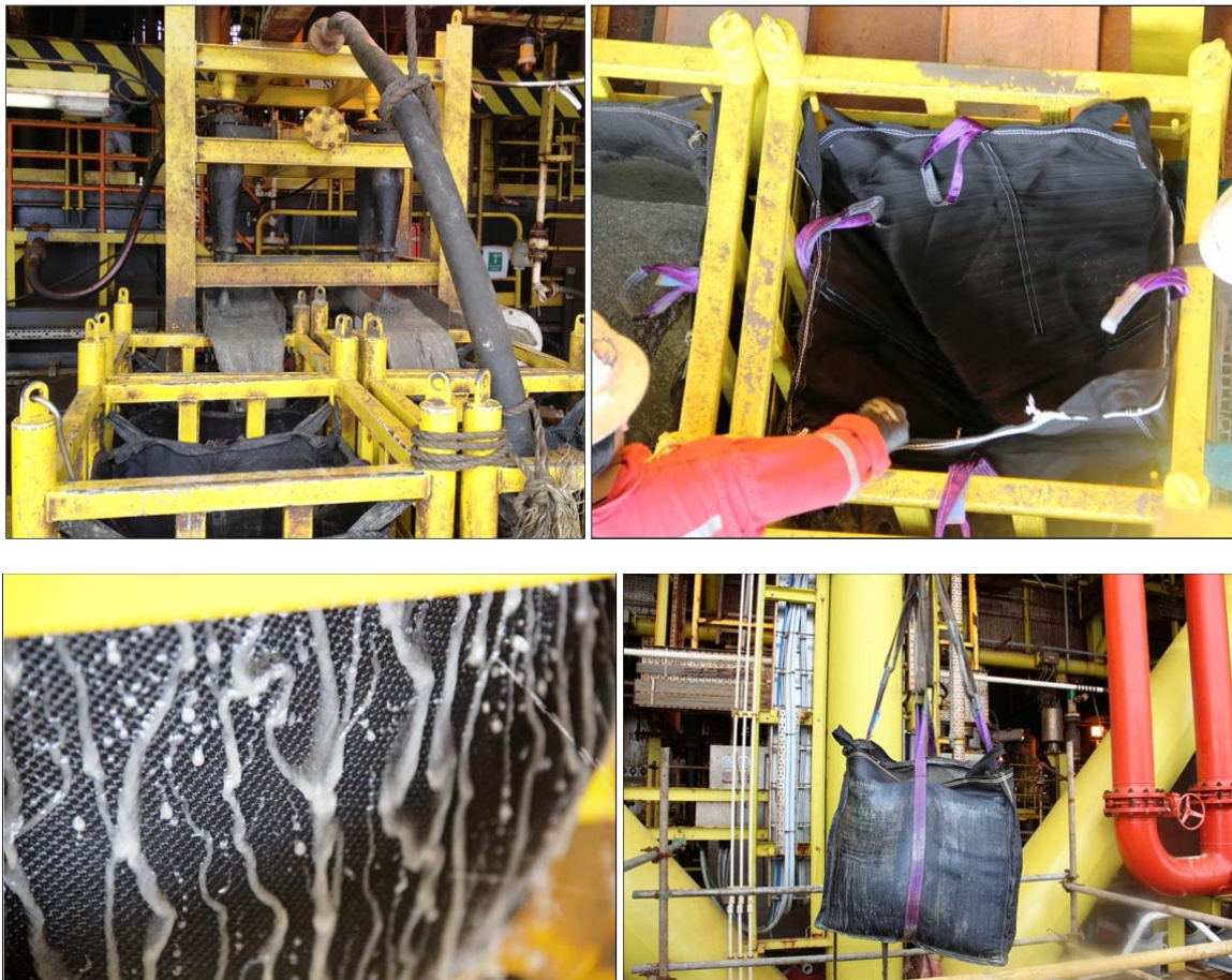
Figure 8 Dewatering and transport station receiving slurry from wellhead desanders on deepwater floating facility. Photos show (top left) bank of hydrocyclones for bulk dewatering, (top right) placement of oleophobic rapid-weep filter bag into holding frame, (bottom left) gravity drain of fluids through filter-bag for final dewatering step, and (bottom right) lift of filled filter-bag for disposal to hopper and eventual landfill.
