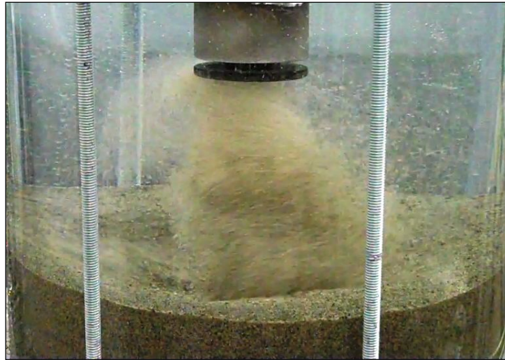
Figure 2 Shielded vortex sand removal demonstrated by cyclonic jetting device within a clear pressure vessel.
