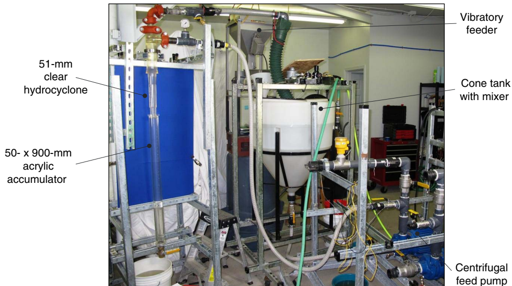
Fig. 6—Experimental flow-loop setup for testing the desander apex-flux rate. The loop consists of a cone tank with a mixer, variable-drive centrifugal feed pump, and a 51-mm-diameter clear hydrocyclone with a cylindrical accumulator.
