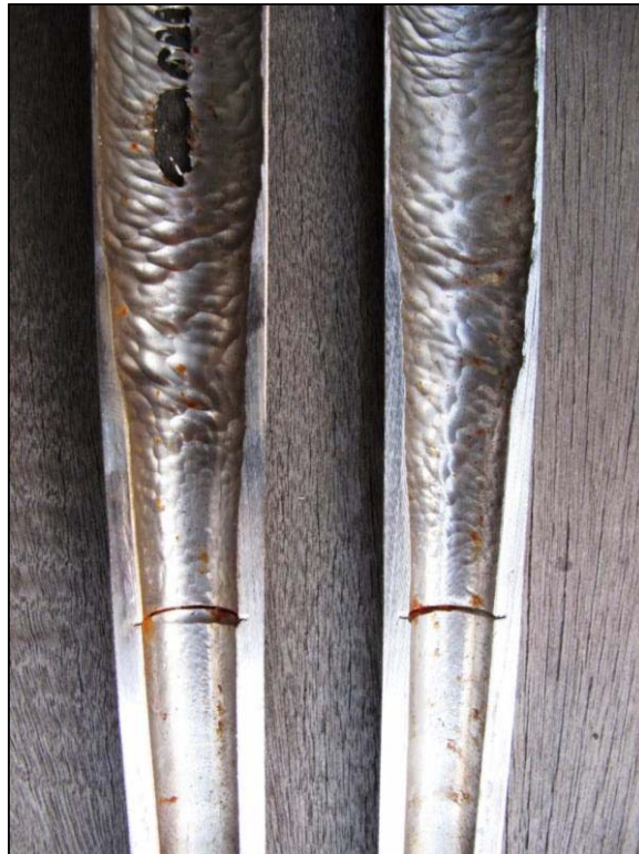
Fig. 5—Erosion marks on a 38-mm-diameter desander, showing premature failure in the cone section caused by a concentration-choked apex. The solids trajectory is from top to bottom. The cone section (top) shows severe wear to failure, whereas the apex (bottom) shows negligible erosion.
