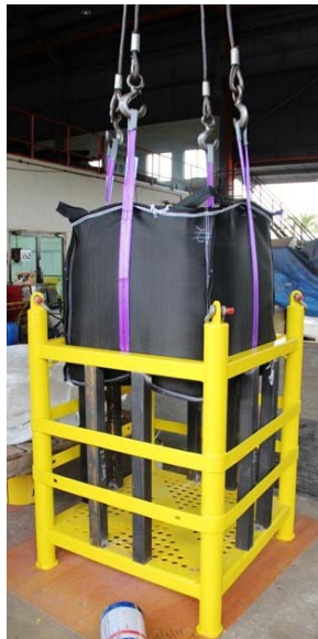
Fig. 5 – Dewatering filter bag (left photo) being lifted from a simple support frame.
