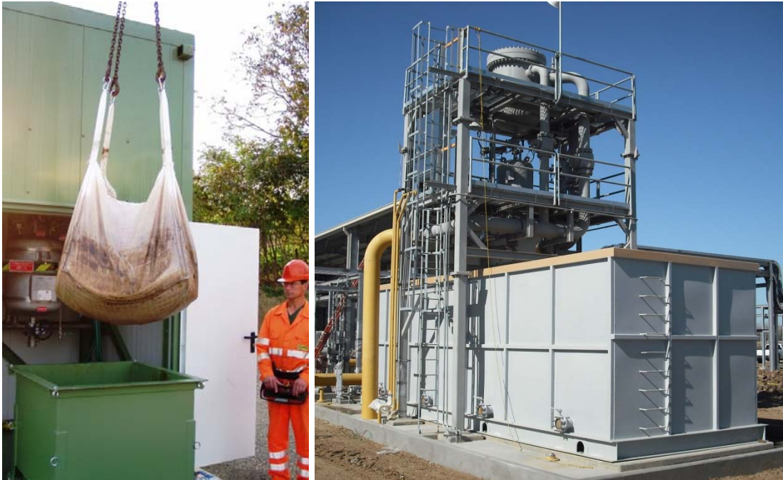
Fig. 8 – (left) Crane lift of a dewatering bag after filling with solids from a multiphase desander and (right) truck roll-off container to collect solids directly discharged from a produced water desander.
