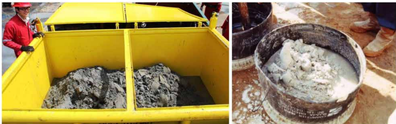
Figure 6—Dewatered sand from offshore Malaysia (left) and onshore Indonesia wells (right).
