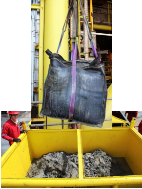
2011 Murphy Kikeh Spar Malaysia Dewatering Bag to Skip
